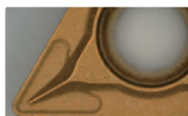
adjust the X-Y metal stage to move the workpiece slowly to generate a stitched image automatically
